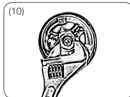
(10) Tighten (10) Overflow Connector using (14) Overflow Connector Screw with adjustable spanner.
