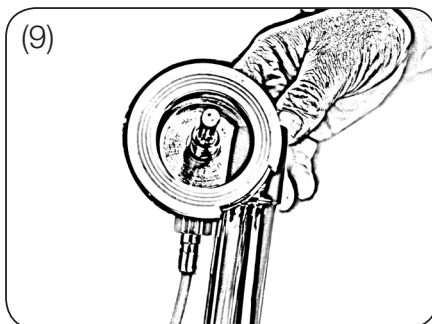
(9) Apply silicone sealant to (11) Rubber Seal and offer to overflow hole.
